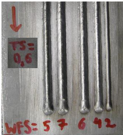
S355, CMT, TS0.5m/min, WFS 2 & 4 & 6m/min
