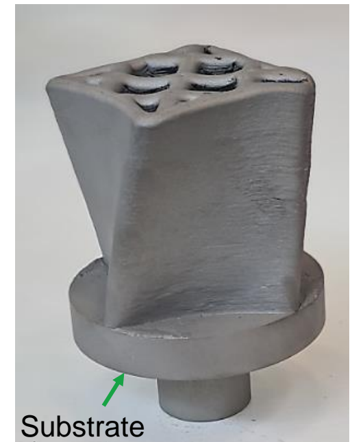
Demonstrator after sandblasting
