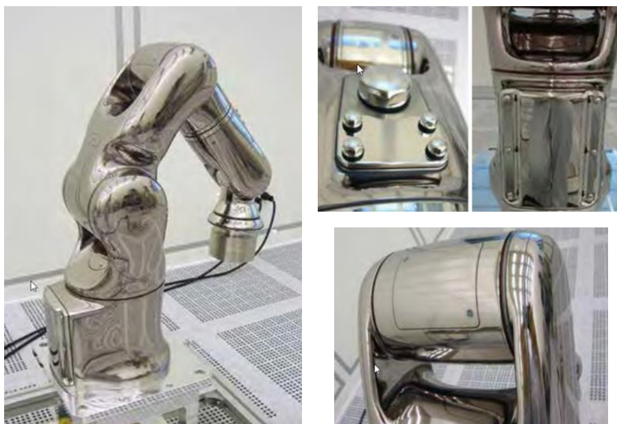
Figure 31 : EHEDG yearbook 2017/2018 - overall hygienic design : screws have been used only at the level of the robot arm to allow pneumatic hoses to be optionally connected for the grippers and on the electronics cover located at the foot of the robot ; cap screws with sealing rings; the joints and lids on the various robot components all have sealed covers to prevent the entry and accumulation of microorganisms and contamination into areas that are difficult to clean
