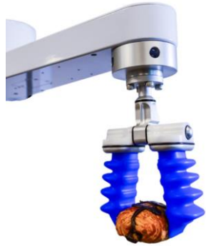
Figure 35 : CIP-able mGrip from Soft Robotic -self-draining
