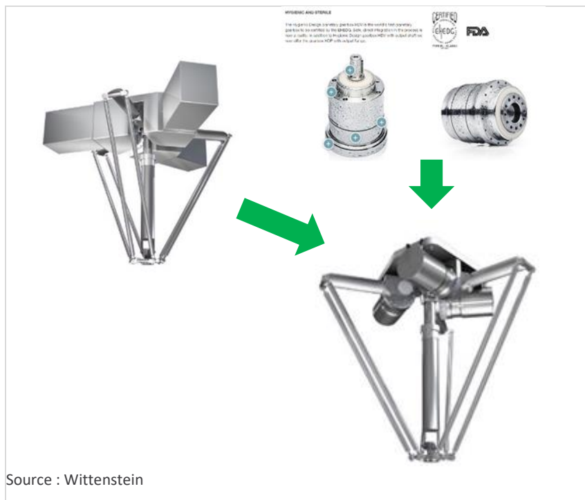
Figure 26 : less pieces, less retention surface thanks to the Hygienic Design motor-gearbox unit. Housing for the drives are not mandatory anymore. The drive is directly integrated in the process.
