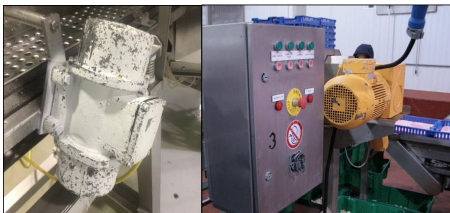
Figure 32: painted equipment on vibrating conveyor belt - cleaning of painted equipment is risky (on courtesy of Frank Moerman)
