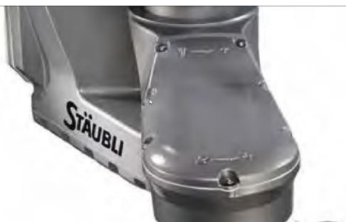
Figure 24. Protected robot against electrical exchanges by physical separation between stainless steel screws and aluminum based structure
