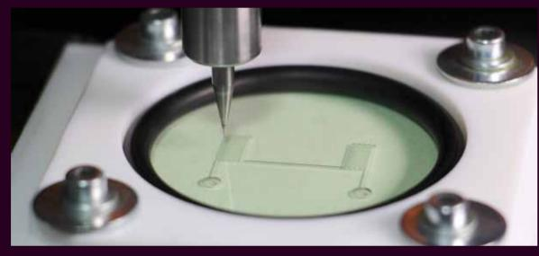
Down to 10 µm min. feature size
