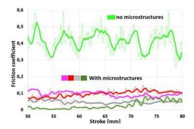
The graph shows that friction decreases when microstructures are applied.
