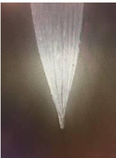
Microneedle, made with a laser-textured mould, in collaboration with KU Leuven Cel Kunststoffen
