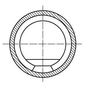
Figure 9.1-1 — Internal stiffening rings with a reinforced cut-out
