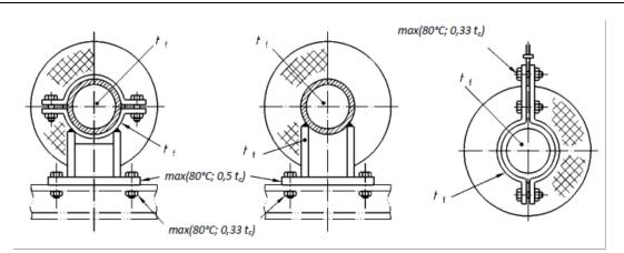
Figure 13.11.2-1 — Support design temperatures inside and outside insulation
