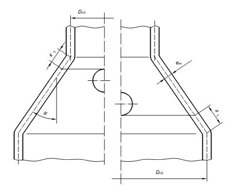
Figure 8.3.2-2 — Opening in a conical shell
