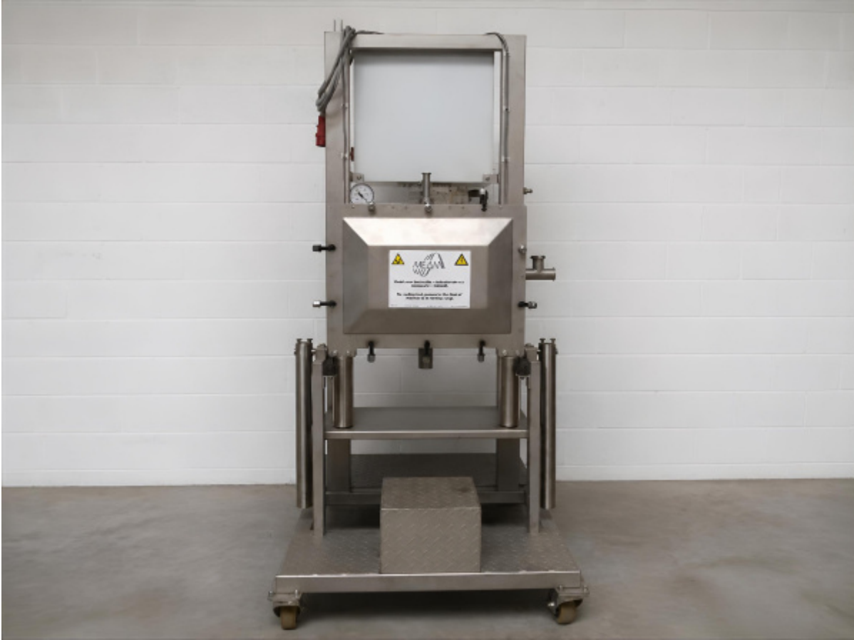
Figure 2. Installation for microwave pyrolysis technology at MEAM.
