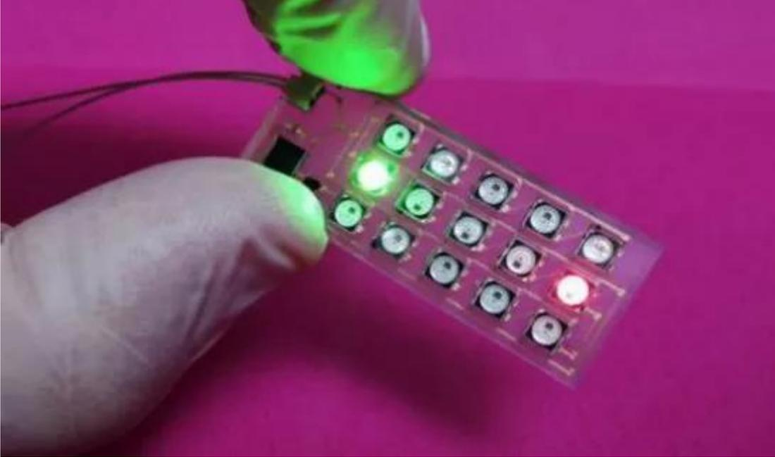
*Figure 4 - Complete and functional 3D-PID component with SMD components integrated on a 3D printed substrate and fed through micro-printed gold circuitry*
