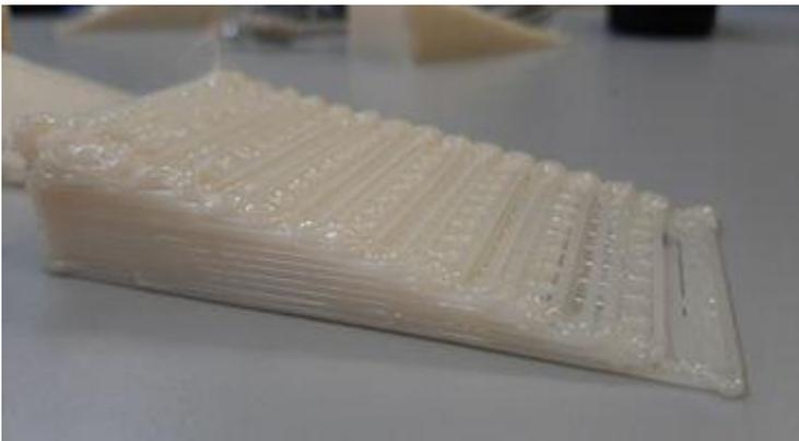
*Figure 2 : Stair stepping effect on shallow angled part*
