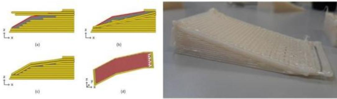
Figure 3 : Non-planar finishing layers
