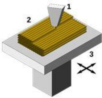
*Figure 1 : Fused deposition modelling*
