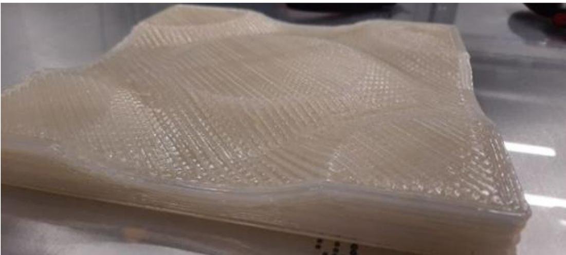
*Figure 5 : Non-planar printed example*
