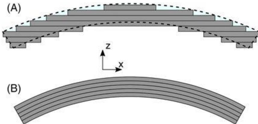
Figure 4 : Conventional vs. conformal layers
