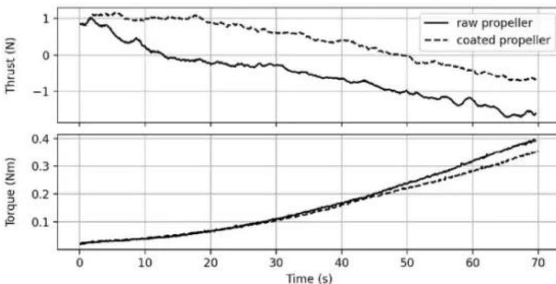
*Figure 3: Comparison of propeller thrust and torque for the coated and non-coated (raw) propeller. Non-coated propeller thrust drops down to zero at  $t = 12s$ , whereas the thrust of coated propeller still is above zero until  $t = 50s$*
