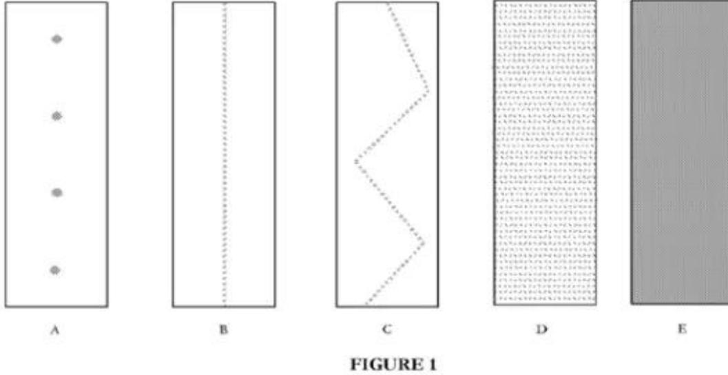
Figure 1 (source: WO2020/128687 A1) illustrates the distance between two consecutive measuring points.
