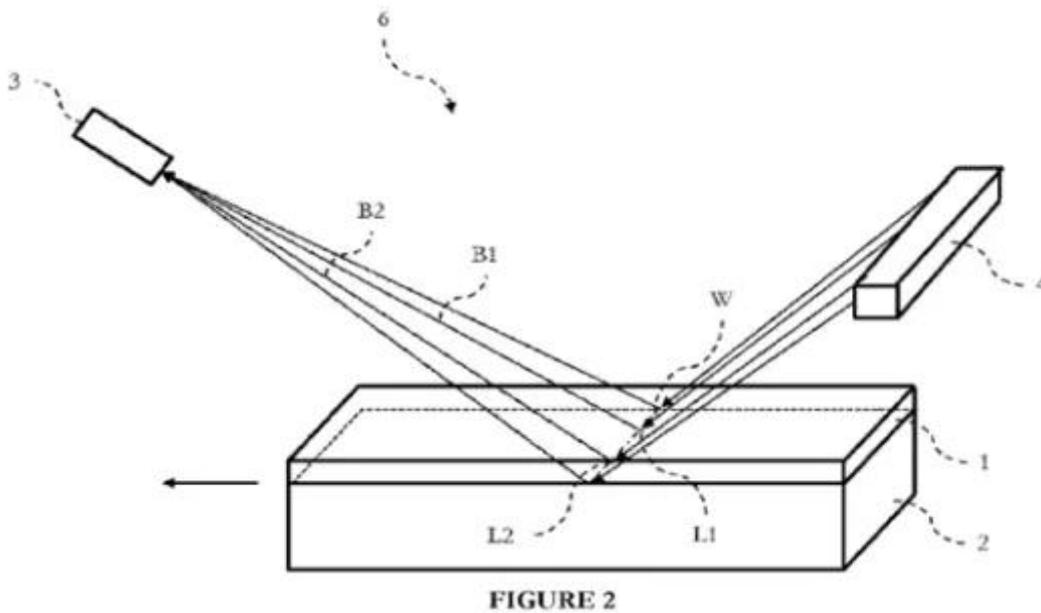
Figure 2 (source: WO2020/128687 A1) shows a measuring setup based on hyperspectral imaging, with which the substrate passing under the setup is imaged over the full width and thus the quality of the coating is monitored over the entire surface.
