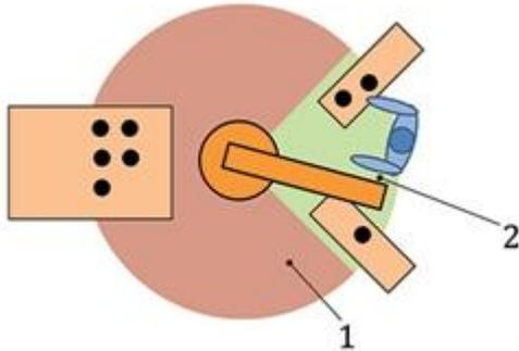
*Diagram of a human-robot collaborative operation, where 1 represents the operating space and 2 the collaborative workspace. (Source : ISO/DIS 10218-2 - previously ISO/TS 15066)*
