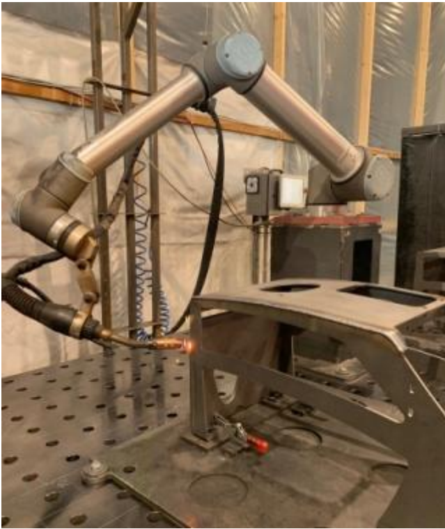
Welding of the hoods by a cobot at Malmar
