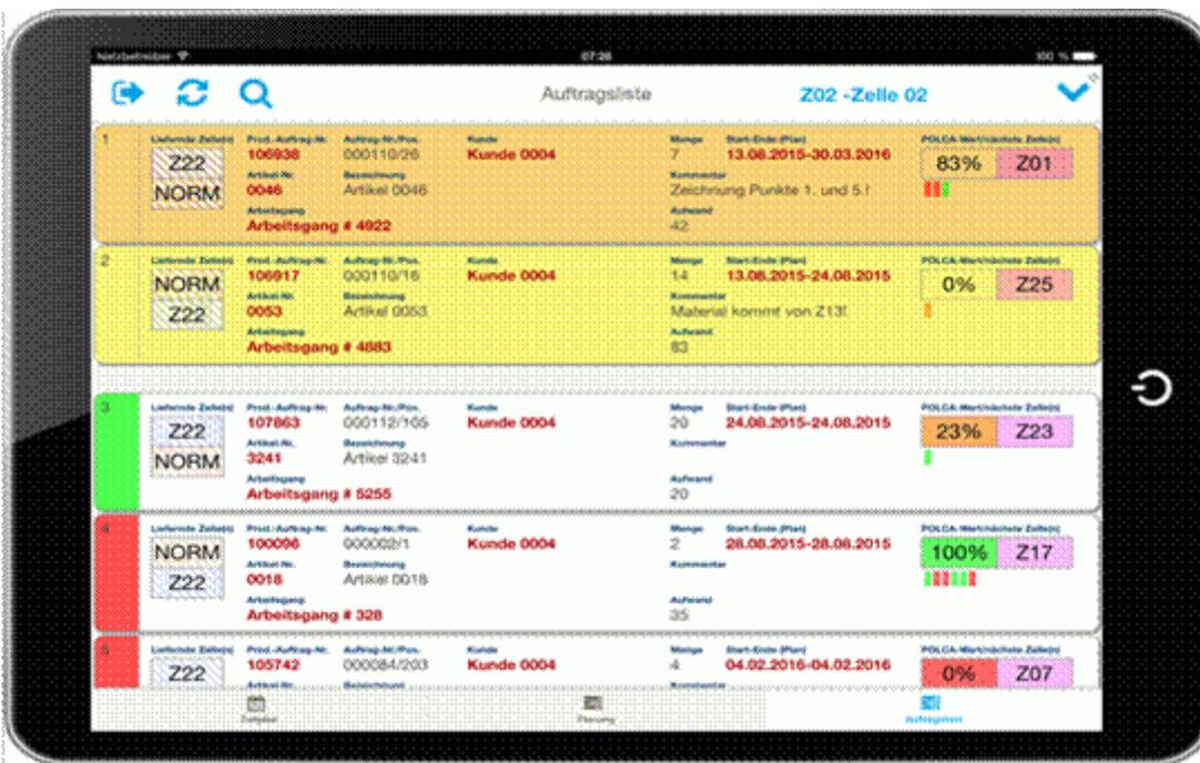
Figure 5: Example of the Timeaxx digital POLCA screen. Availability of cards is displayed by a percentage on the right side of the screen.
