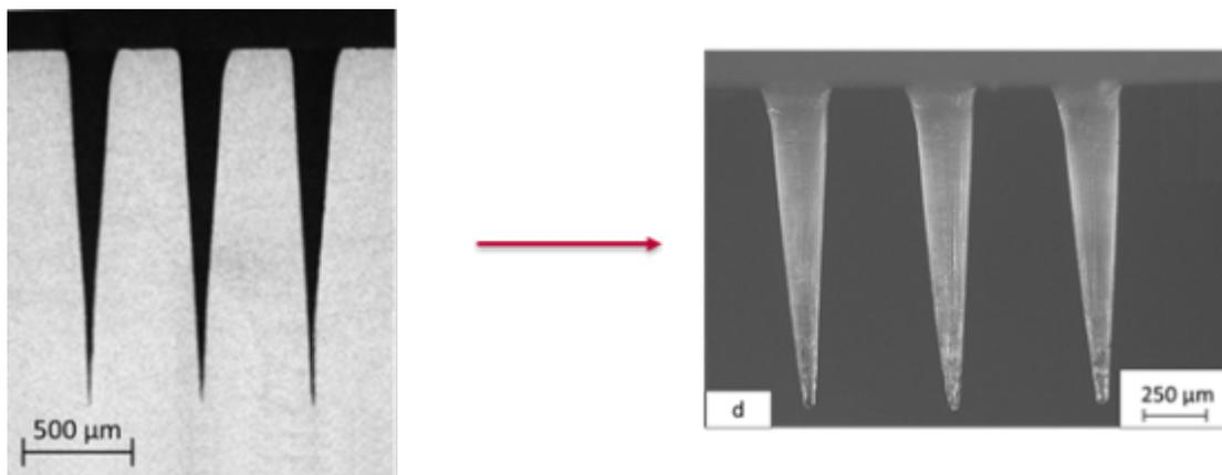
Figure 2: Mould (left) and needle (right)
