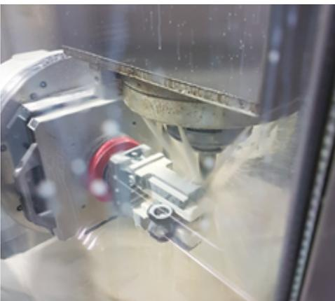
Precision machining of features on the AM part is usually a process with very high stakes as the part would be scrapped if it does not meet the final tolerance requirements. Enough knowledge and expertise is required to be able to successfully machine complex parts built with AM technologies.
