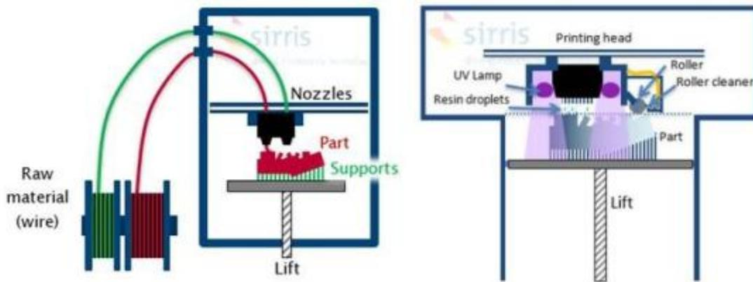
Left: material extrusion principle, right: material jetting principle
