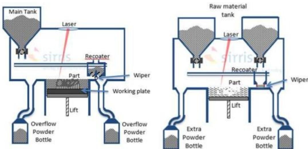
*Powder Bed fusion (laser metal) principle (left), selective laser sintering principle (right)*
