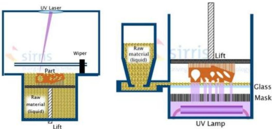
*Vat Photopolymerization principle, with laser (left) and with DLP (right)*
