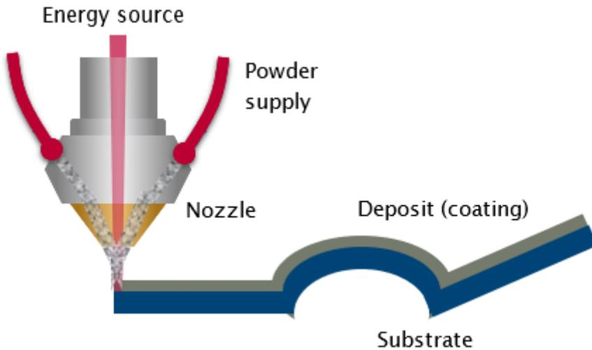
*Direct energy deposition principle*
