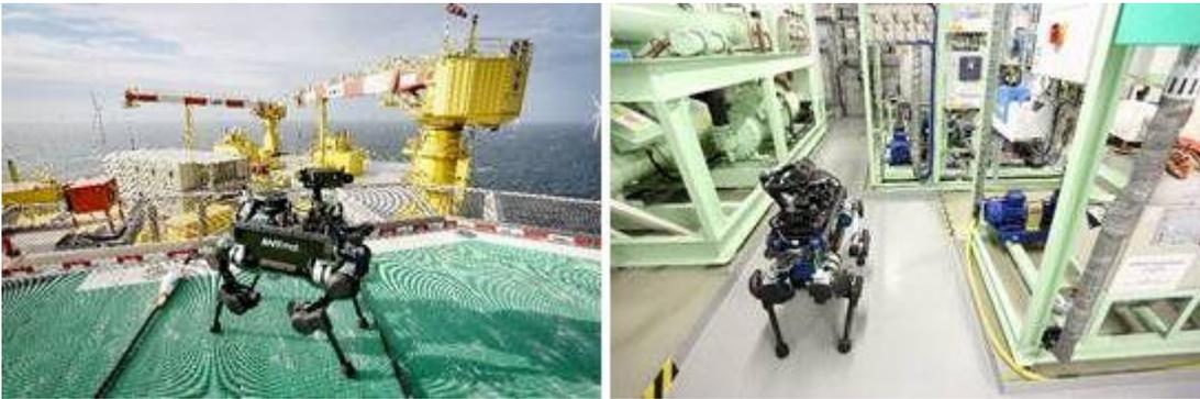
*Proof of concept of an inspection tour with the ANYmal-robot in an offshore transfo station*
